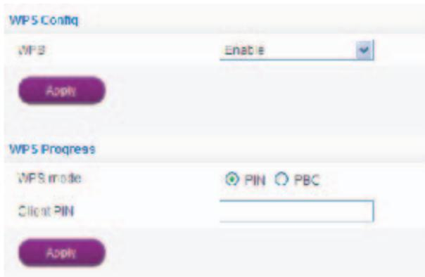
The screenshot shows the 'WPS Config' interface after being updated. The 'WPS' dropdown menu is now set to 'Enable'. Below this, there is a purple 'Apply' button. A new section titled 'WPS Progress' is visible, containing 'WPS mode' with two radio button options: 'PIN' (which is selected) and 'PBC'. Below the radio buttons is a text input field labeled 'Client PIN'. A second purple 'Apply' button is located at the bottom of this section.
