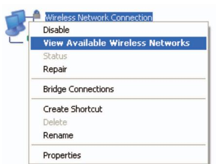
NOTE: Please set the client to obtain an IP address automatically, and the client will get an IP address like “192.168.0.100”.
