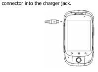
2. Connect the charger to a standard AC wall outlet. 3. Disconnect the charger when the battery is fully charged.
