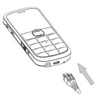
Remove the charger from both the AC outlet and the phone once the charging is completed.
