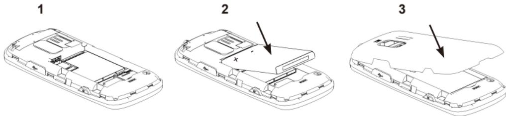
1. Insert the battery by aligning the contacts (1) and then gently press it down until it clicks into place (2).
