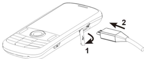
1. Pull the rubber USB cover out of the USB port and move it out of the way.
