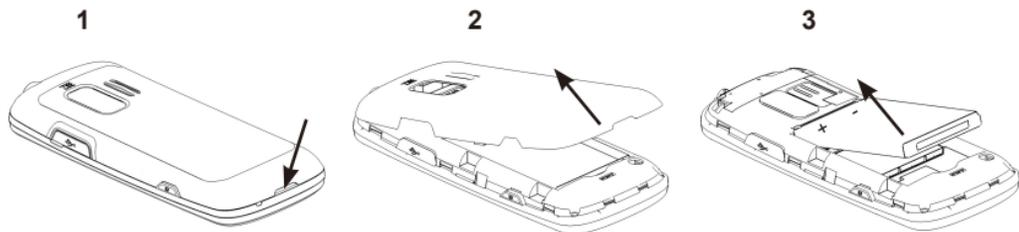
1. Insert your fingernail into the back cover slot on the bottom of the phone and lift off the back cover (1) (2).
