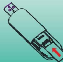
3. If necessary, insert the microSD card into the microSD card holder until you hear a click. Make sure the metal contacts of the memory card orientated as shown in the right picture.
