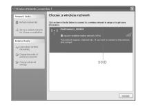
There will be a pop-up window to require the password. Check the label on your device to gain the SSID and preset password information. Please do remember the new password when you change the password by selecting Settings > Wi-Fi Settings > Security after logging in the WebGUI Configuration Page. You can restore the device to the factory default settings in case you forget it.
