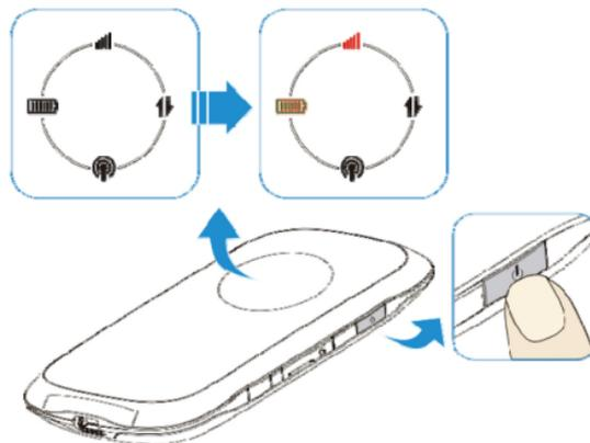
2). Use your normal Wi-Fi application on the client to search the available wireless network, when the Wi-Fi LED is blinking.
